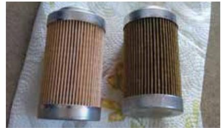
New filter on left. Filter on right is after 2,000 miles. Problems were traced to contaminated fuel.
