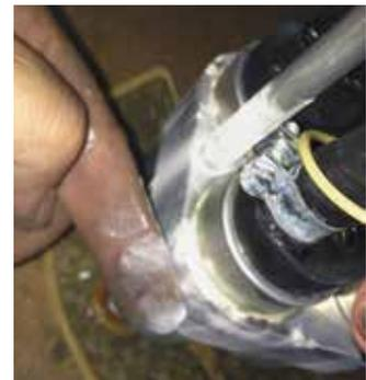
Fine white powder on a non-anodized aluminum bracket reacting with E85.
